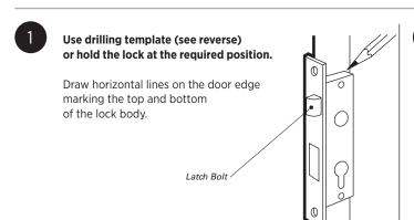
Mark a vertical line at the centre of the door edge between the two horizontal lines.
