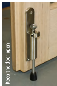
Foot Operated Door Catch Door Mounted Height/Width: 145x27mm Throw: 55mm
