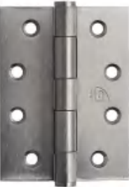
Brushed Stainless Steel 304 SSS 45105 85x60x2mm Fixed Pin 45107 100x60x2mm Fixed Pin 45108 100x75x2.5mm Fixed Pin 45109 100x100x2.5mm Fixed Pin 45115 85x60x2mm LoosePin 45118 100x75x2.5mm LoosePin
