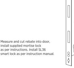
Measure and cut rebate into door, install supplied mortise lock as per instructions. Install SL36
