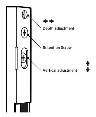
Adjust the striker to secure the door using the adjustment screws, the adjustments can be up and down by loosening the vertical adjustment screws and the depth by loosening the retention screw and turning the depth adjustment screw.
