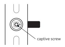
Using an allen key, remove captive screw from inside and remove the factory fitted long handle. Install small handles using new screws supplied, new screws have fresh thread lock included.
