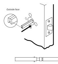
Fit rubber O-ring into slot mid way down spindle.
