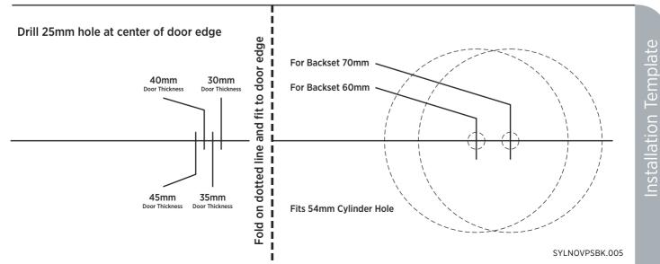
DRILL POINT FOR STRIKE Drill 25mm hole 13mm deep in door jamb a. Locate the strike cutout at drill point **CAUTION:** To assure proper lockset function, hole in jamb must be drilled a full 13mm deep.
