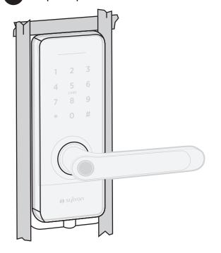
Using a non-marking or painters masking tape, tape the case to the door around 3 sides to secure to the door, leaving the base exposed.
