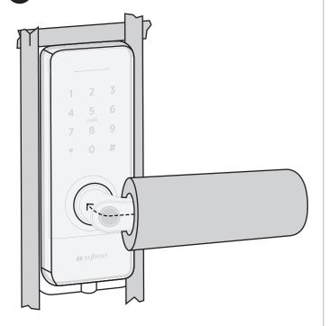
Slide the sleeve over the lever handle completely until it butts up against the clear case, creating a good seal.
