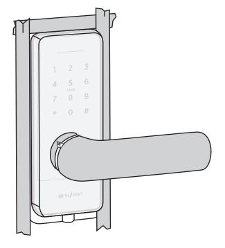
Using the supplied cable tie, firmly secure the sleeve onto the lever handle.
