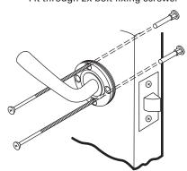
Fit both handles onto spindle.
