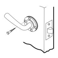
Fit cover plates over handles, ensure notch is at the bottom.
