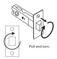
Fit spindle through latch.
