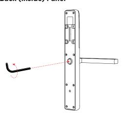
1. Using an allen key, remove screws from the inside of the handle
