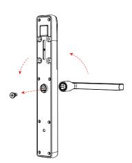
2.Remove and rotate the handle to the left or right depending on handing direction.
