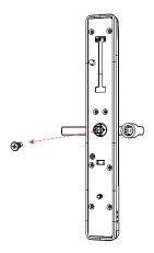
2.Remove and rotate the handle to the left or right depending on handing direction.
