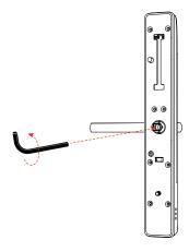
1. Using an allen key, remove screws from the inside of the handle
